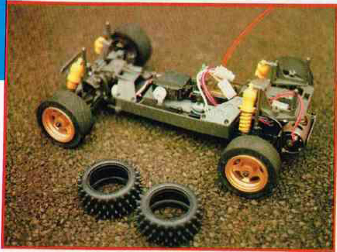
Above and left, clearly shown in these photos are the suspension ride height adjustment system. Left the Thunderbird comes complete with two sets of tyres, on and off road.
